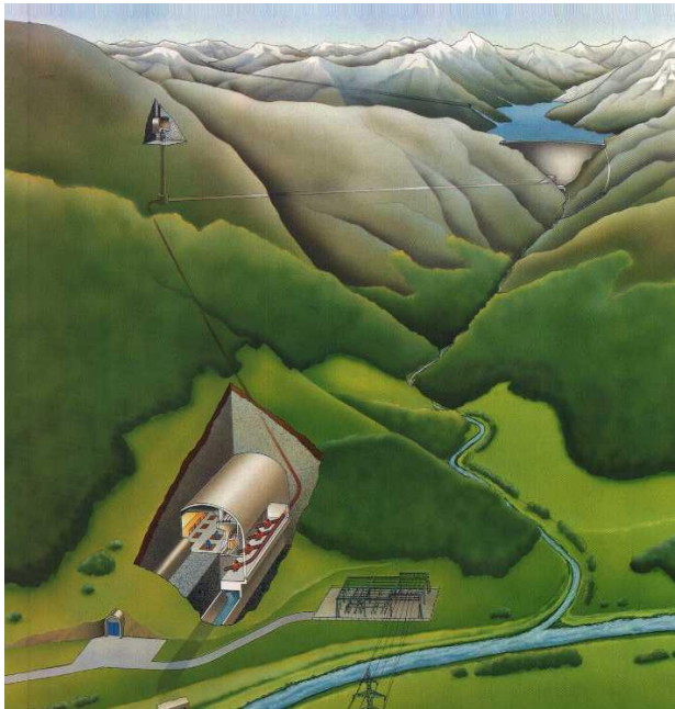
Figure 2-2 Overview of a storage hydropower plant (VSE-INFEL) with main elements starting from reservoir fed eventually by diversion tunnels from neighbouring catchment, arch dam, power intake, pressure tunnel, surge tank, pressure shaft, underground powerhouse, tailrace channel and switchyard.
